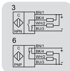
Capacitive Sensors S26 with hemispherical active surface for level control of products with a dielectric constant  $\epsilon_r$  as of 1,1. Products can be:
