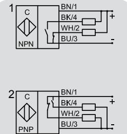
Capacitive Sensors S26 with hemispherical active surface for level control of products with a dielectric constant  $\epsilon_r$  as of 1,1. Products can be:
