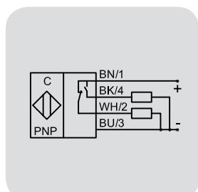
Capacitive Sensors S26 with hemispherical active surface for level control of products with a dielectric constant  $\epsilon_r$  as of 1,1. Products can be:
