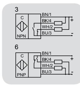
Capacitive Sensors S26 with hemispherical active surface for level control of products with a dielectric constant  $\epsilon_r$  as of 1,1. Products can be:
