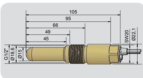
Capacitive Sensors S26 with hemispherical active surface for level control of products with a dielectric constant  $\epsilon_r$  as of 1,1. Products can be:
