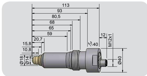
Capacitive Sensors S26 with hemispherical active surface for level control of products with a dielectric constant  $\epsilon_r$  as of 1.25. Products can be:
