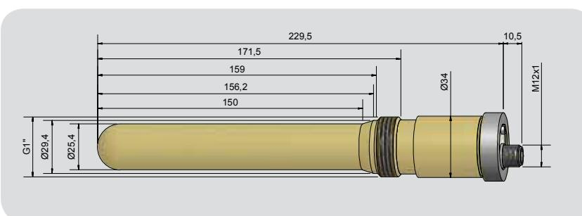
Capacitive Sensors S26 with hemispherical active surface for level control of products with a dielectric constant  $\epsilon_r$  as of 1,1. Products can be:
