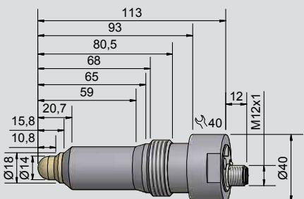
Capacitive Sensors S26 with hemispherical active surface for level control of products with a dielectric constant  $\epsilon_r$  as of 1.25. Products can be:
